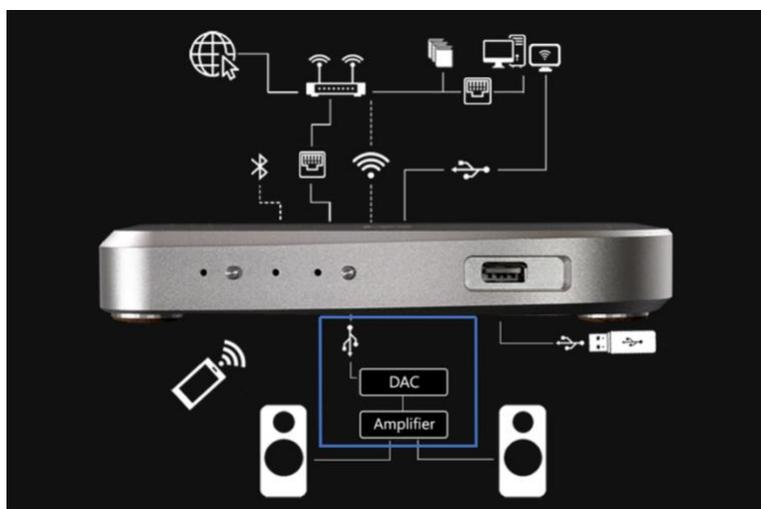
It has only one output, the USB Type A connector (10) on the back panel. This can be connected to any USB equipped DAC or DAC/Amplifier. A USB cable with a Type A connector for the LINK end and either a Type A or B connector for the DAC should be used.
