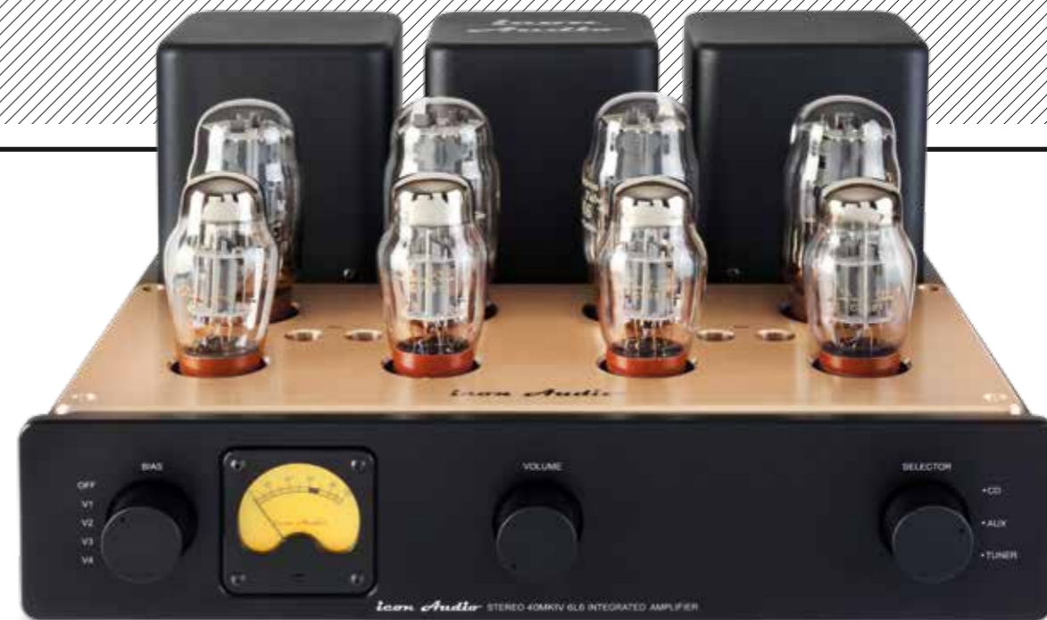
LEFT: Stripped of the Stereo 40 MkIV's features including the Triode/Ultralinear mode switch, speaker/headphone selector and socket, on/standby and tape monitor, the 'new' ST40's fascia sports a simpler array of volume, input selection and valve bias knobs
