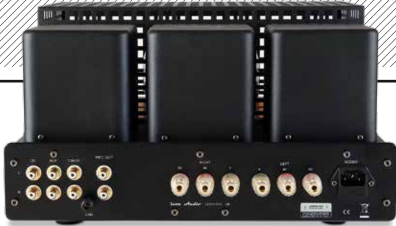
ABOVE: Two output transformers [far left/right] have dual secondaries feeding the 4 and 8ohm speaker outlets. Three line ins (no MM/MC) and a tape loop are included
