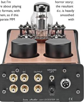
Our rear shots shows gold plated, phono socket inputs and outputs, a ground lift switch to avoid hum, and a ground terminal. The circular canisters are screening cans around the input transformers.
