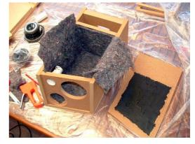
impossible. If you can't achieve correct positioning take off the clamps, separate the pieces and use a wet rag to clean off the glue before you try again. They should match up perfectly but minor imperfections in the joints can be corrected at the sanding phase.
