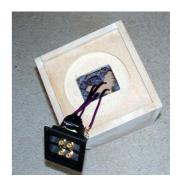
holes gradually so that the terminal block goes right into the cut out in the base. Once in place drill pilot holes and screw the terminal block in place with four #6 19mm screws.
