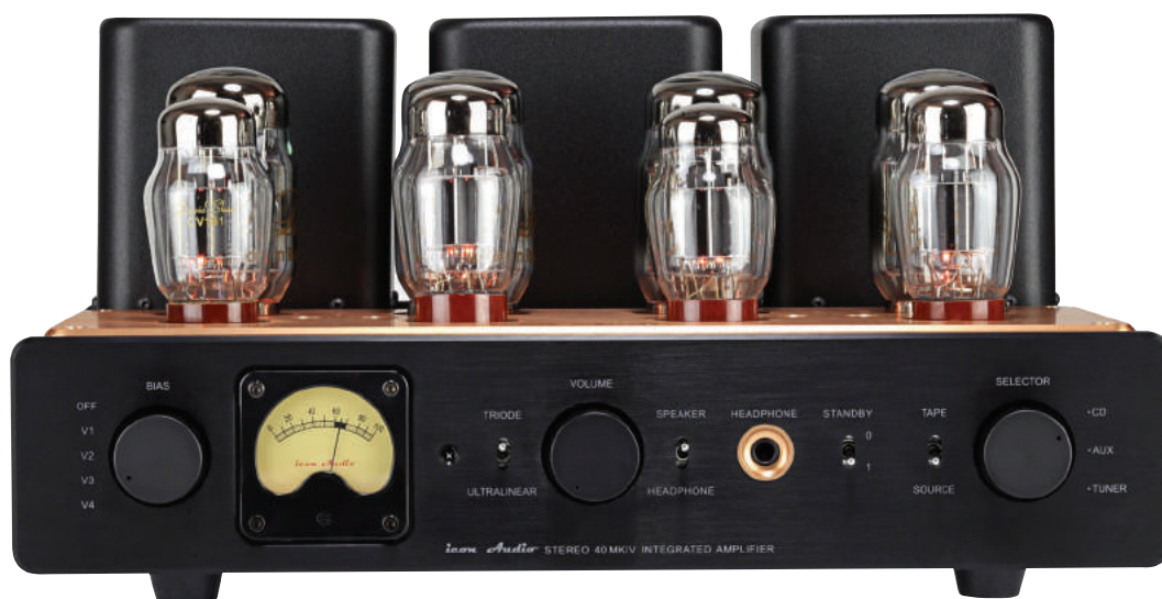
At left the input bias adjust selector for V1-V4 output valves, bias adjusted to put the needle into the black sector on the meter scale. Then a Triode / Ultralinear lever switch, volume control (centre) headphone socket, Standby switch, Tape switch and rotary input selector at far right.
