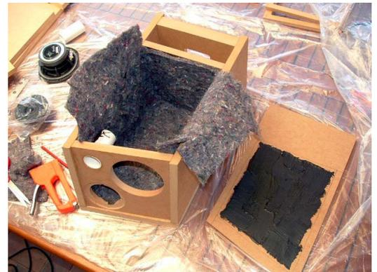
7. Once the glue has set you can apply more glue liberally to all the joins inside the chamber to ensure an airtight seal.
