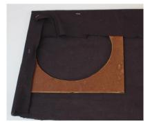
15. At this point your speaker enclosure is finished except for the fact that there are two raw timber edges on each side. The faces are coated with a thin layer of hardwax oil and I recommend sanding that off so that you finish up with bare timber all over. I applied three coats of satin enamel to the prototypes which gave a very nice finish.
