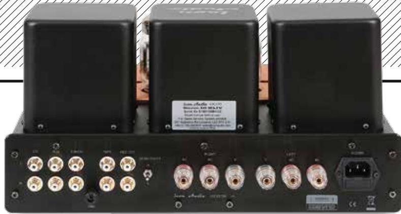
**ABOVE:** Two output transformers [far left / right] have dual secondaries feeding the 4 and 8ohm speaker outlets. Three line ins and a tape loop are included (no phono) while the 'H'/'L' toggle offers a choice of High or Low sensitivity [see boxout, p59]
